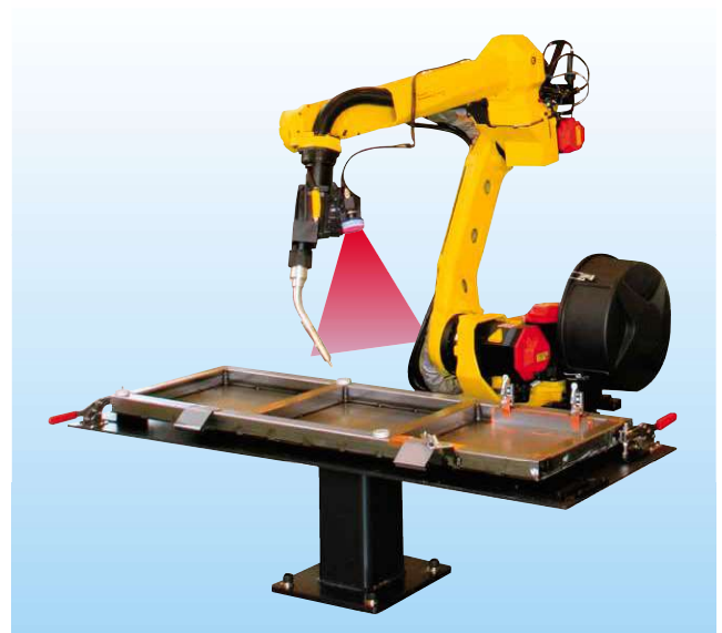
Architectural part arc welding with i RVision
