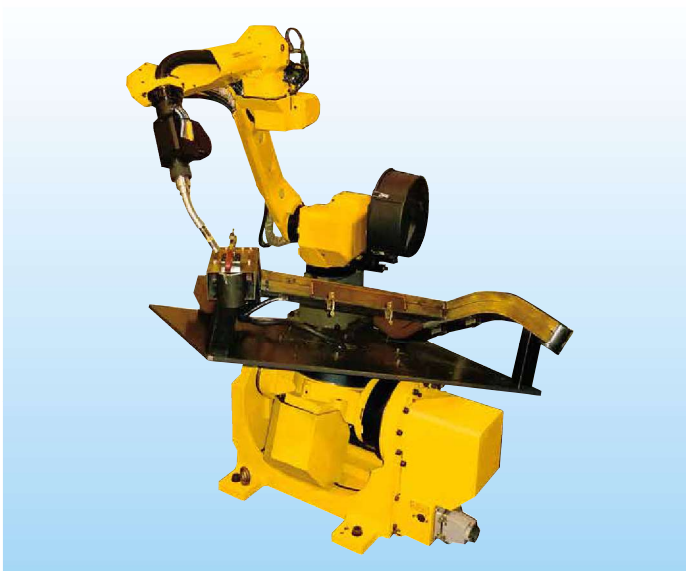
Automobile part arc welding with Servo Torch
